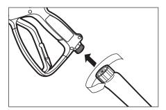
**Step 2** Attach high pressure hose to trigger gun.
